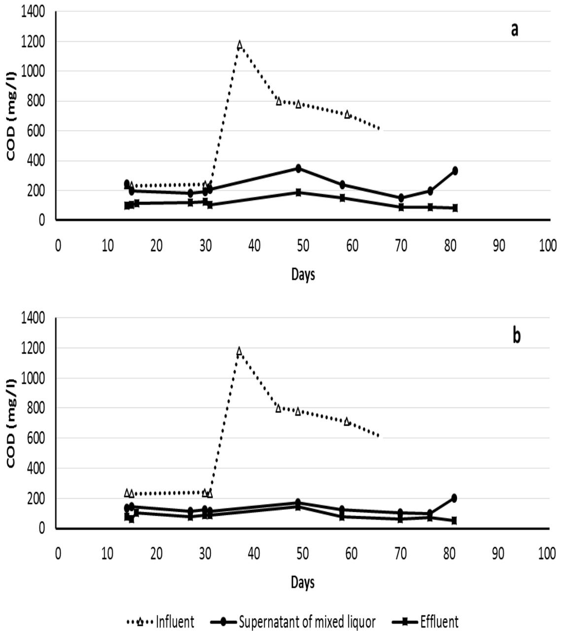
Fig. 11 - COD of influent, effluent and the supernatant of the mixed liquor of activated sludge in (a) the acidic reactor and (b) the neutral reactor.
