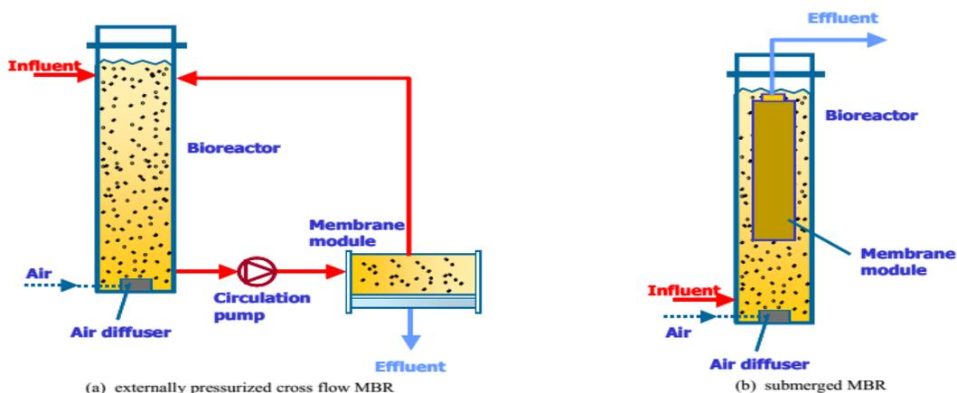
Figure 2: Different configurations of MBR process (Garbhani and Farajnezad, 2012).
