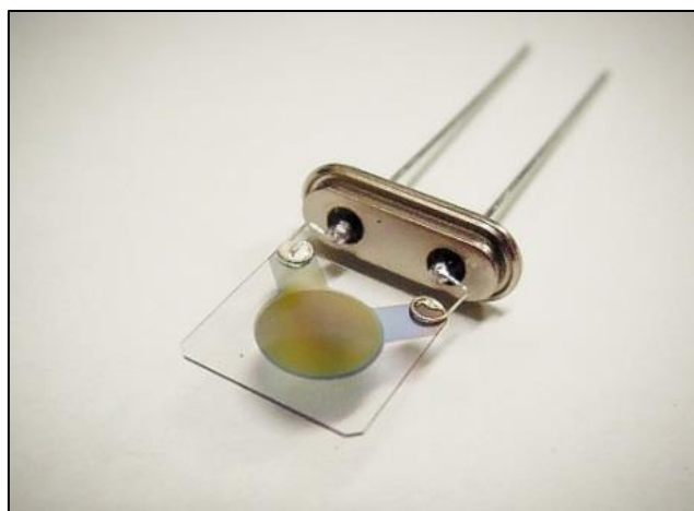
Figure 2-6. Quartz crystal microbalance manufactured.
