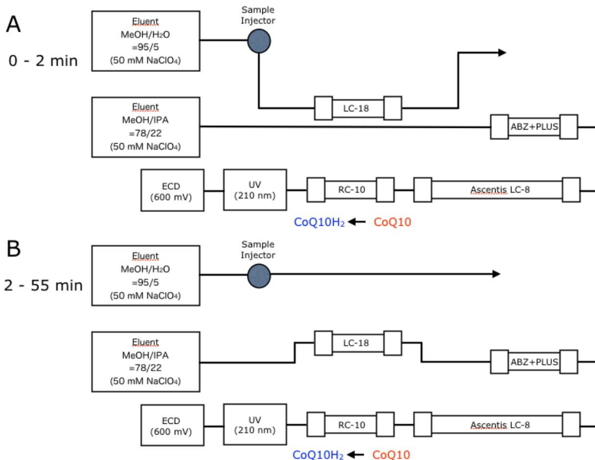
Fig. 1 Column switching system for the analysis of CoQ10H<sub>2</sub> and CoQ10 in human CSF.
